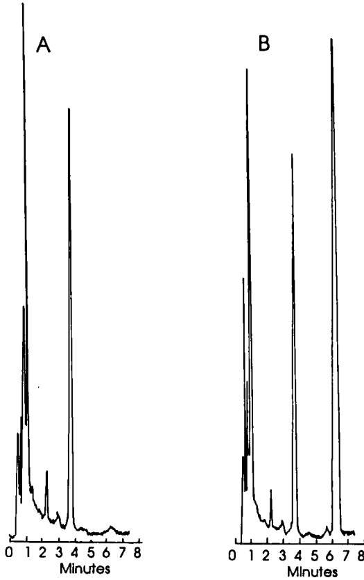
Figure 2. Representative chromatographic traces showing: A, extract of blank water sample showing only the internal standard, dipentyl phthalate, and B, extract of water sample spiked with 0.1 \mu\text{g/mL} methoprene.
